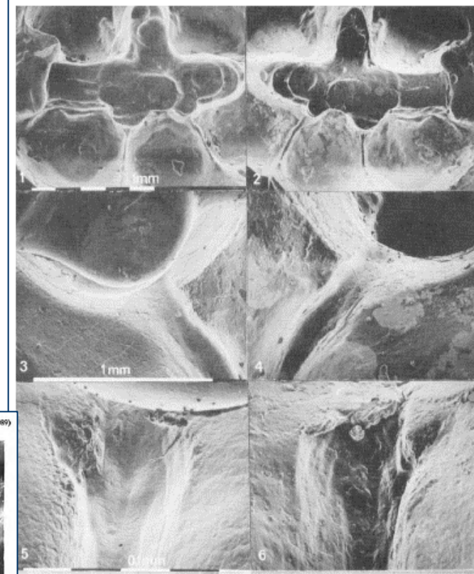
Figs. 1-6. SEM micrographs of a class-II cavity preparation made in 1979. Figs. 1, 3, and 5 are 10-year-old negative replicas made of a condensation silicone elastomer, while Figs. 2, 4, and 6 are 10-year-old positive replicas made of epoxy. Magnification: Figs. 1 and 2, ×10; Figs. 3 and 4, distobuccal fissure on Fig. 1, ×75; Figs. 5 and 6, mesiobuccal fissure on Fig. 1, ×200. The light gray zones on the surface on the epoxy replicas are presumably caused by a chemical interaction between the impression material and the epoxy material at the time of casting.
